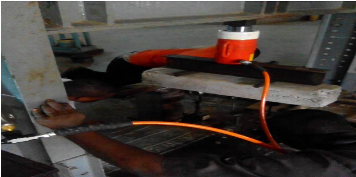
Figure 1. Flexural strength setup for beam under third-point loading
