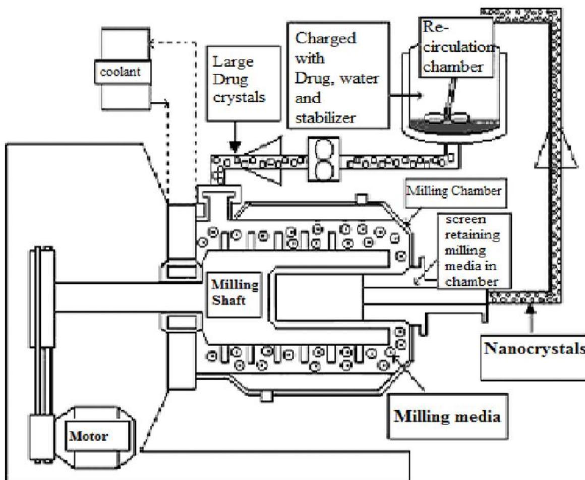
Fig.4- Schematic representation of media milling process
