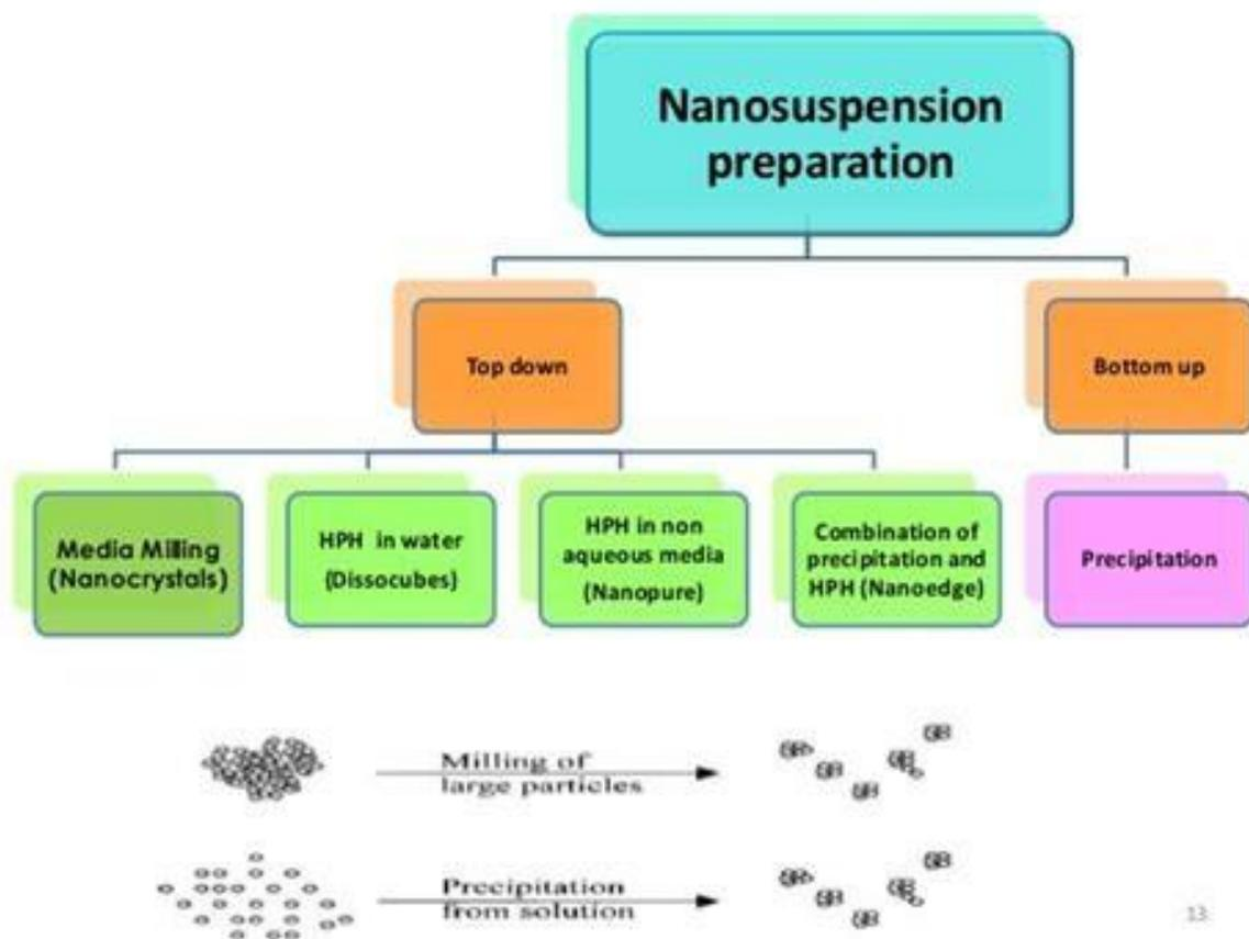
Fig .2- Method of Preparation of Nanosuspension
