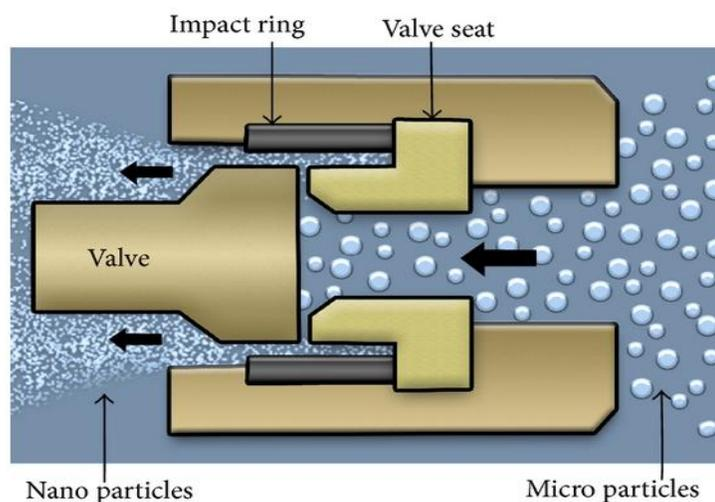
Fig.3-High-pressure homogenizer process
