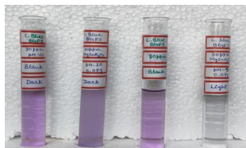
Photo 5: Effect of light with respect to Dark condition and UV condition on photocatalytic degradation of Coralene Blue BGFS in 300 minutes
