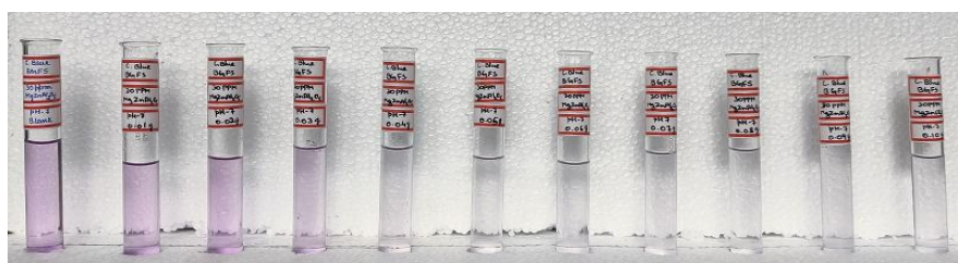
Photo 2: Effect of catalyst concentration on Coralene Blue BGFS dye at 300minutes=30 ppm, pH=7
