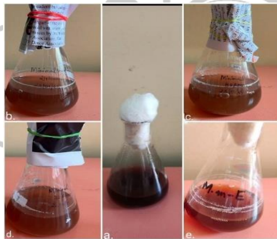
Fig. 5: A. Untreated melanoidin; Melanoidin decolorization by Priestia aryabhatai mvy-004 at 37°C in MSM at different incubation time B. 24 hrs C. 48 hrs D. 72 hrs and E. 96 hrs
