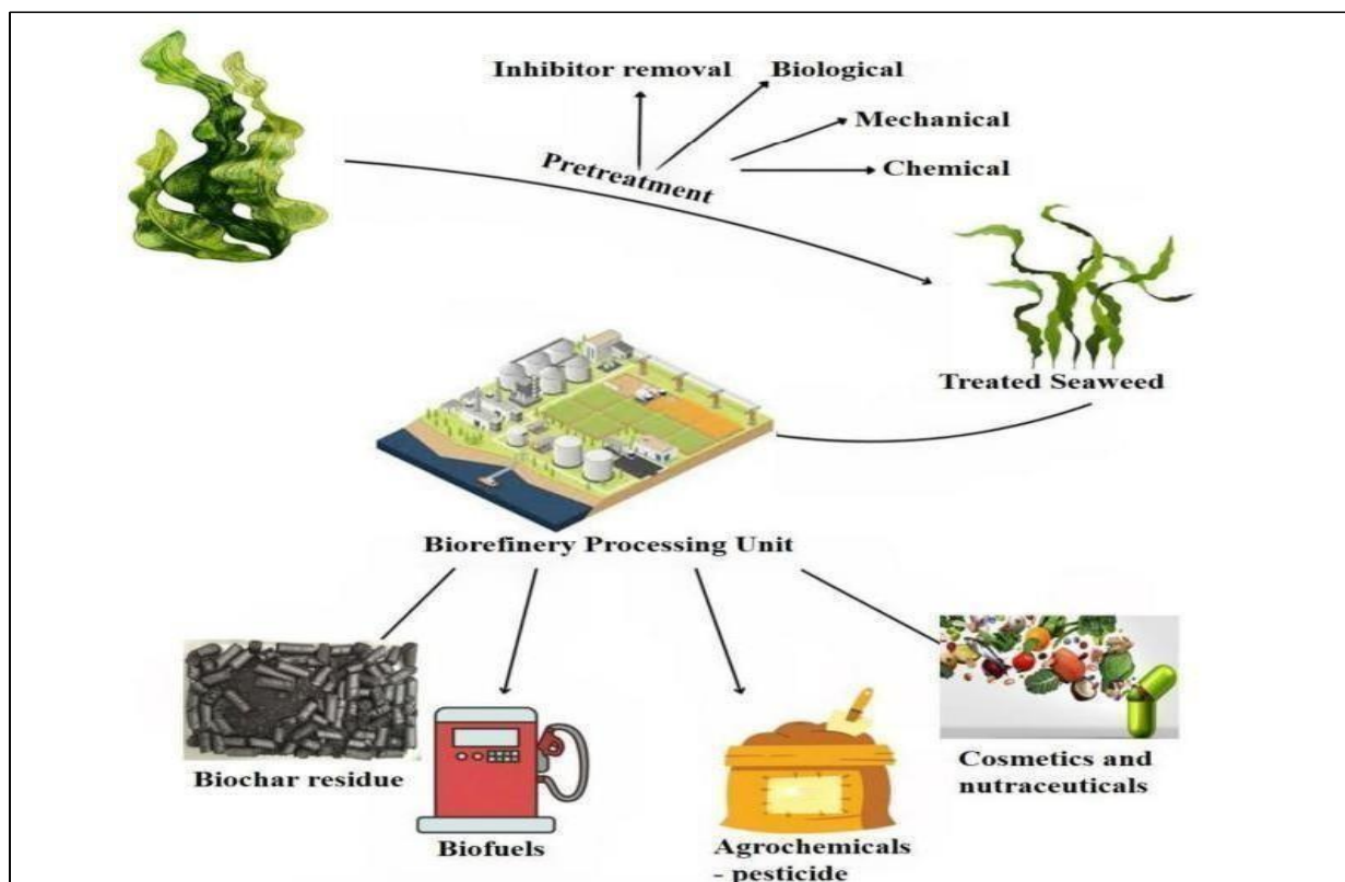
Figure No. 3 Biorefinery Process of Pesticide Production from Marine Seaweeds
