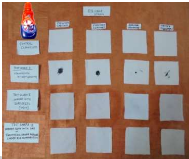
(B) Washing results with Jasmine Oil driven Nanoparticles
