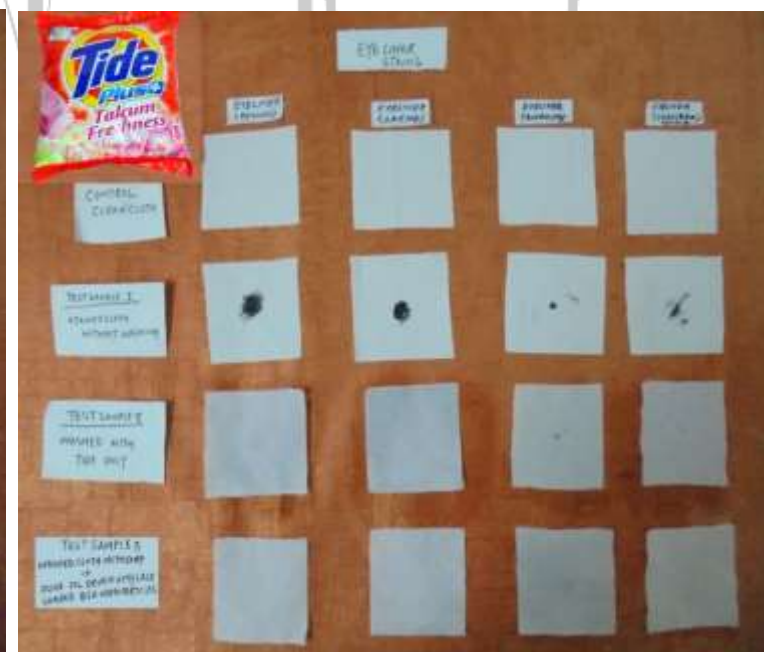
(D) Washing results with Olive Oil driven nanoparticles
