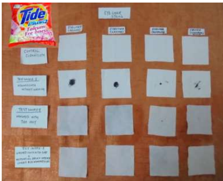
Figure 4 : Washing results of Eye-liner stained cloth with Tide Plus alone and Tide Plus with amylase loaded nanoparticles prepared with different emulsifiers- Almond oil, Jasmine Oil, Mustard Oil and Olive Oil
