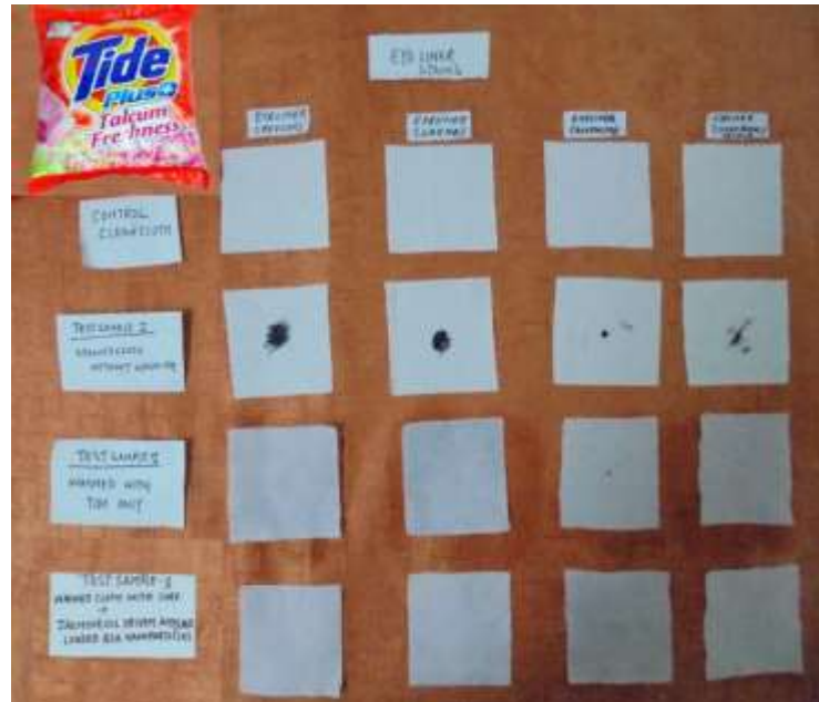
Figure 4 : Washing results of Eye-liner stained cloth with Tide Plus alone and Tide Plus with amylase loaded nanoparticles prepared with different emulsifiers- Almond oil, Jasmine Oil, Mustard Oil and Olive Oil
